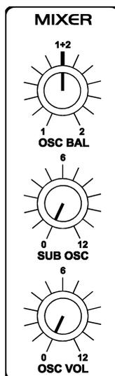
You have already come across two parameters of the MIXER section: **OSC BAL** determines the mix ratio between Oscillators 1 and 2; in the left half of its control range, **OSC VOL** determines the master volume of the oscillator mix. In the right half of the control range from the center position to the far right, OSC VOL increases the saturation intensity when a SATURATION curve has been activated.
