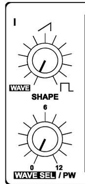
To this point, we have turned our attention exclusively to sound-shaping functions and have always started with the same basic material: a so-called sawtooth wave. This waveshape is especially well-suited as a neutral starting point as it contains all of the so-called natural scale of overtones, which give the filter plenty of quality material to work with.
