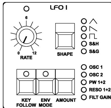
Start with the usual basic sound configuration or chose a modified sound to suit your taste. Locate the **RATE** pot in the LFO 1 section of the control panel. The RATE pot is equipped with an LED that indicates the speed of the LFO as well as its waveshape. Turn the RATE pot and check out how the flash of the LED indicates the change of pace as you rotate the pot.
