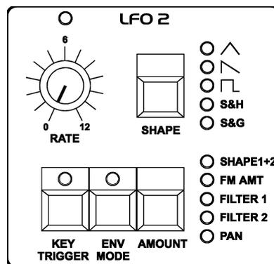
The design of the second LFO is essentially the same as the first, so we'll spare you the repetition of details. The only two differences are immediately apparent when you look at the control panel: SHAPE 1 and 2 are available as a joint modulation target; the FM intensity, filter frequencies and the Panorama position can be manipulated individually. And instead of the KEY FOLLOW function of LFO 1, here you have an option entitled **KEY TRIGGER**. It works like this:
